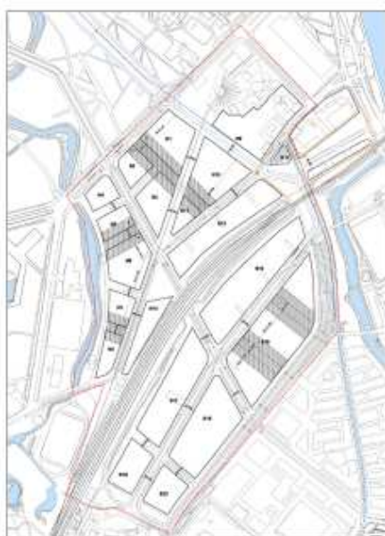
Figure 1.29: Plan of development plots showing limits of deviation and minimum dimensions for roads
