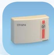
SILENT-100 12V must be wired to a safety isolating **transformer CT-12/14** which must be located out of the reach of the water spray or person using a bath or shower. The transformer is IP21, class II insulation and protected by fuse. Also available, **Transformer CT12/14 R**, supplied with adjustable run-on-timer between 1 to 30 minutes.
