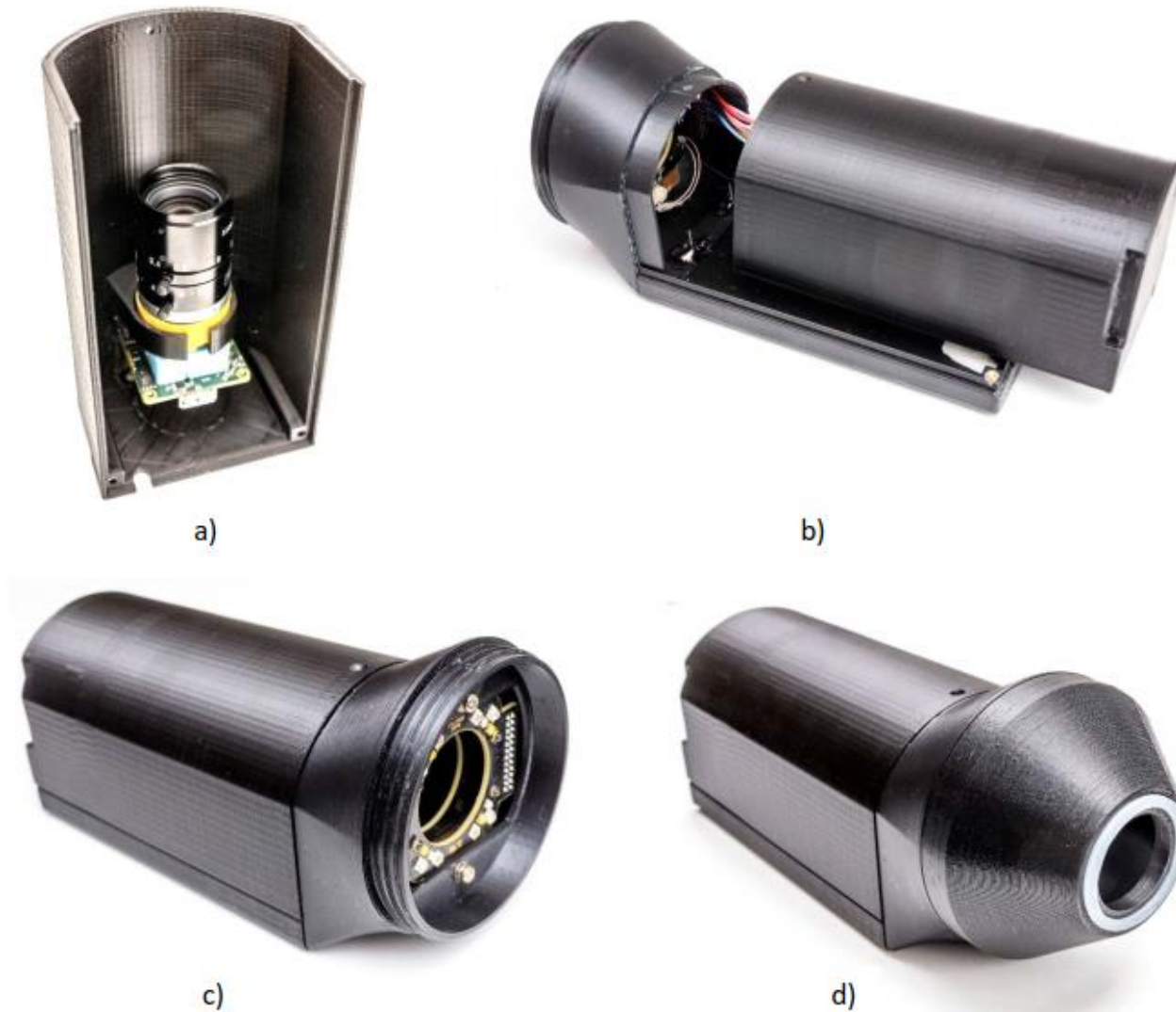
Figure 9. Full prototype printout. Uppercase with lens and camera attached (a), back view with opened upper case(b), attached case without LED holder cone (c), assembled case (d).
