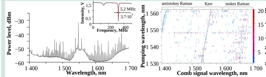
**Kerr comb generated with 166 μm sphere.** 32 different C-Band channel frequencies were pumped inside the WGM microsphere. Only 12 Channels generated Kerr comb lines. Using a 1547.72 nm laser light a comb was obtained spanning from 1400 – 1700 nm with FSR of (3.17±0.08) nm.
