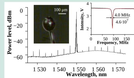
**Kerr comb generated with 170 μm sphere.** A comb like structure with comb spacing (3.14 ± 0.04) nm was observed, the radius of the resonator was calculated as (84 ± 1) μm.
