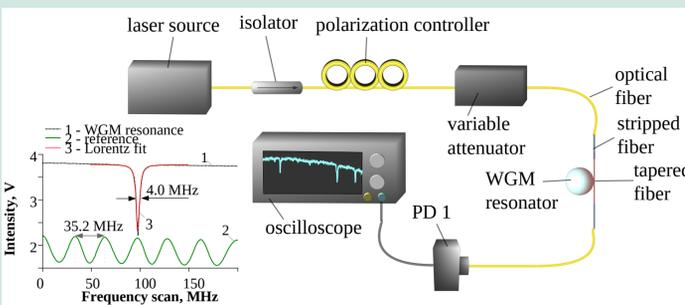
**Characterizing WGM Resonators.** The resonators were characterized by measurement of the Q factor. The measurement system was set up using a 1550 nm laser which was scanned to excite the WGM resonances. A photo-diode was used to record the transmission dips which corresponded to the resonances. Additionally, interferometer fringes from a 3 m long optical fiber were used as a reference signal.
