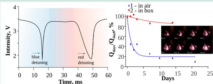
**Non-linearity and Q degradation.** In silica WGM microresonators it was possible to observe nonlinear effects while measuring the Q factor. Depending on the scanning direction of the laser the WGM resonance dips were compresses for blue detuning or broadened for red detuning due to the nonlinear effects. The effects are dependent on the Q factor. If the resonator aged the nonlinear effects became less pronounced.
