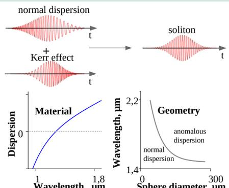
**Dispersion VS Kerr effect.** Both the material and geometry dispersion of the WGM microresonator contribute to the total dispersion.
