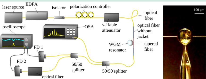
**The figure shows a basic set-up scheme for Kerr Frequency comb generation.** A tunable 1550 nm laser was amplified and coupled inside a silica microsphere using a tapered fiber. Two photo-diodes were used: one to monitor the transmission signal and detect the WGM resonances and other to identify which WGM resonances generated the frequency comb. OSA was used to record the generated comb signal.
