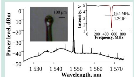
**Kerr comb generated with 120 μm sphere.** A comb like structure with comb spacing (4.31 ± 0.10) nm was observed, the radius of the resonator was calculated as (61 ± 1) μm.
