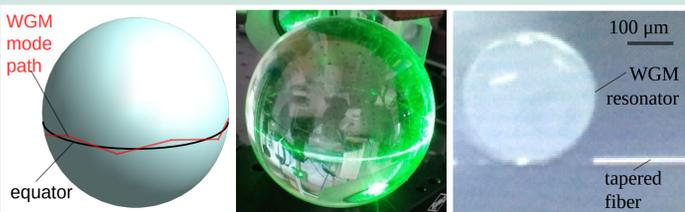
**WGM Resonators.** The light waves inside a WGM resonator are almost perfectly guided round by repeated optical total internal reflection. To couple the light inside the microsphere a coupling element like a prism or tapered fiber is necessary.
