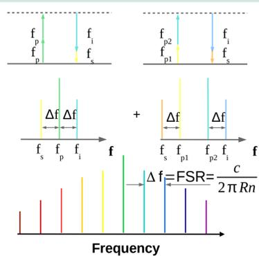
**FWM VS losses.** The degenerate FWM excites an equidistant signal and idler lines and both regular and degenerate FWM generate new comb lines.
