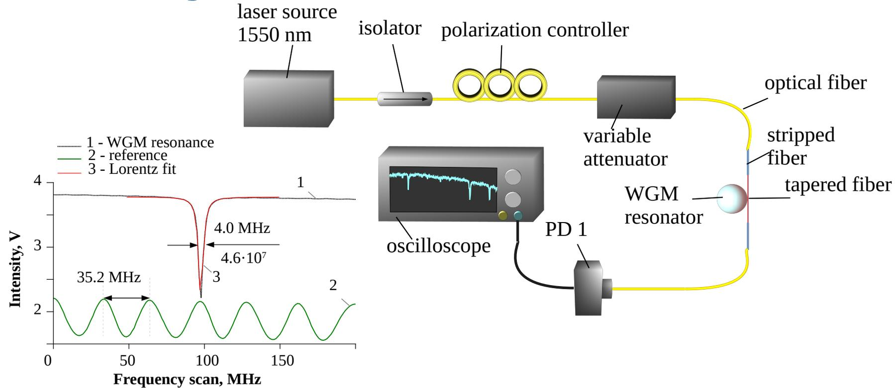
The resonators were characterized by measurement of the Q factor.
