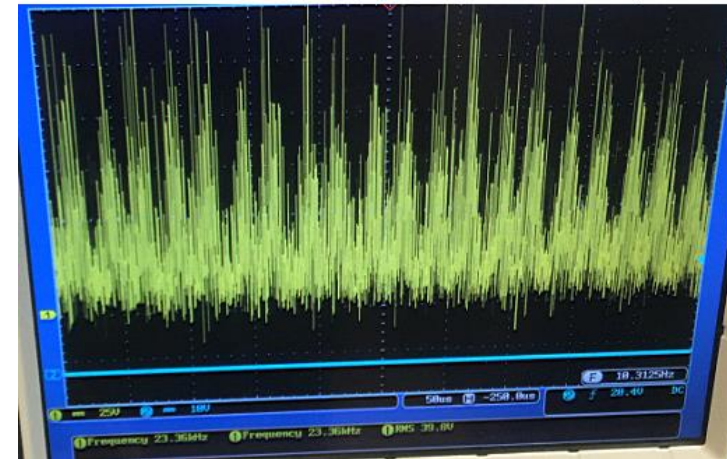
Thermal instabilities on oscilloscope
