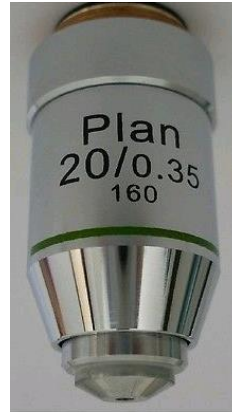
20 x biology microscope objective from Ebay and Levenhuk130 [1.3 Mp] astronomy CMOS camera
