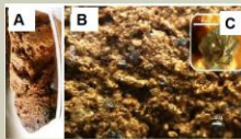
Fig. 4. Micrographs of the surface of ceramic beads sampled from the Column III (A, B, C) at the end of the experiment. Blue crystals on the beads in Column III were formed during wastewater treatment.
