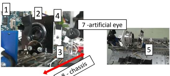
1- CCD matrix with electric circuit, 2- focusing optics, 3- servo motor, 4- semitransparent mirror, 5- IR LED, 6- artificial eye, 7- system stand with moveable chassis.
