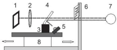
1- CCD matrix with electric circuit, 2- focusing optics, 3- servo motor, 4- semitransparent mirror, 5- IR LED, 6- accommodative stimuli, 7- subjects eye, 8- system stand with moveable chassis.
