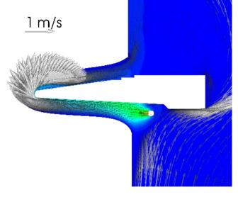
3D inductor shape and non-symmetric dopant inlet
