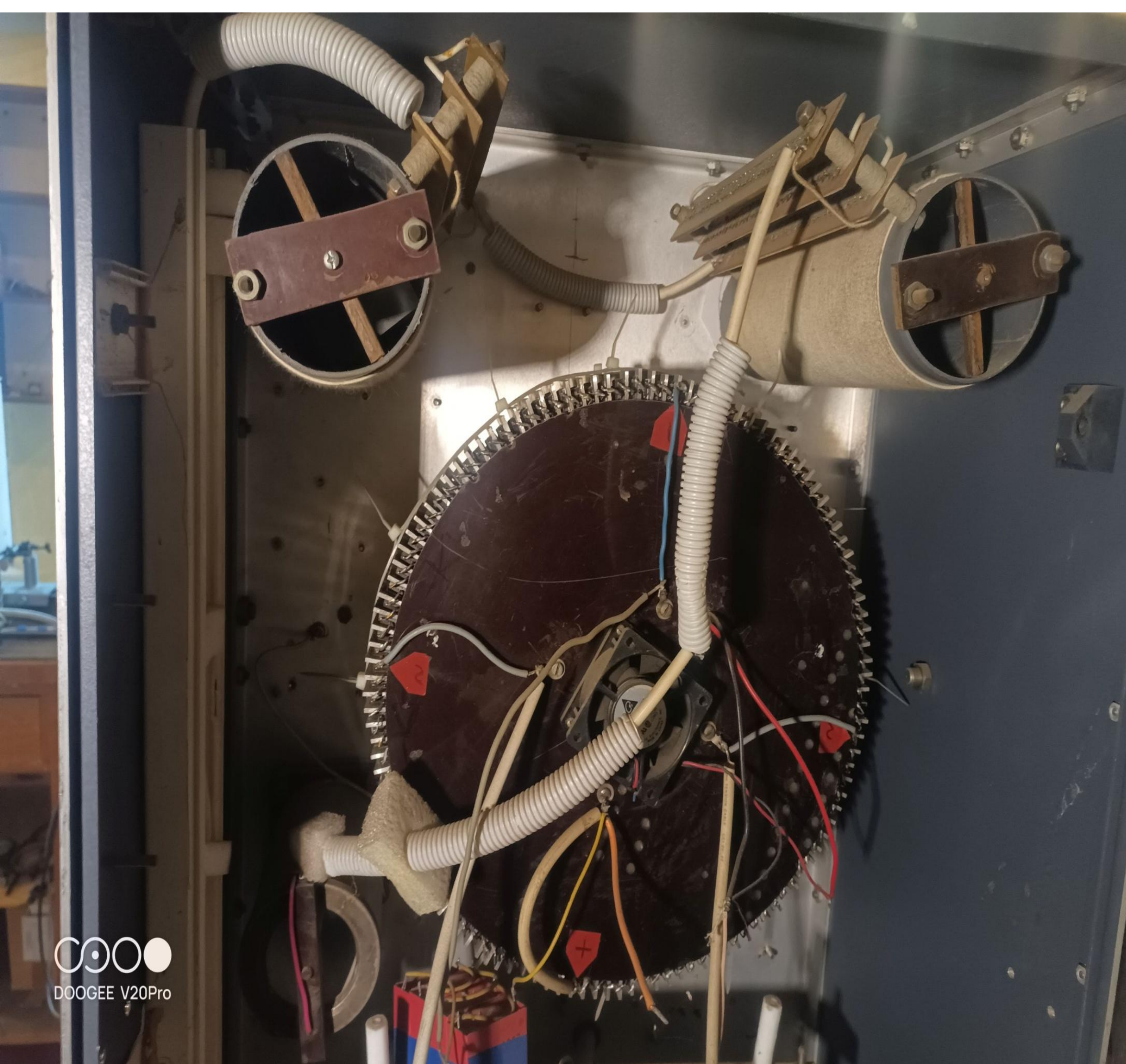
Upper part – serial two aperiodic coils Lower part – 30 kV 5 A Graetz bridge
