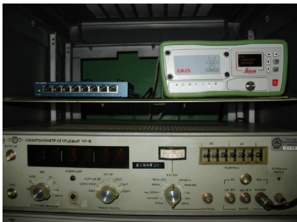
Picture 23. Geodetic GNSS receiver Leica GR25 capable of tracking all major GNSS systems: GPS, Glonass, Galileo, Beidou installed at Geodynamical station Riga
