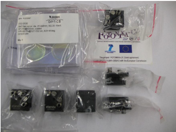
Picture 39. Set of components for optical coude (flat mirrors and mirror holders).
