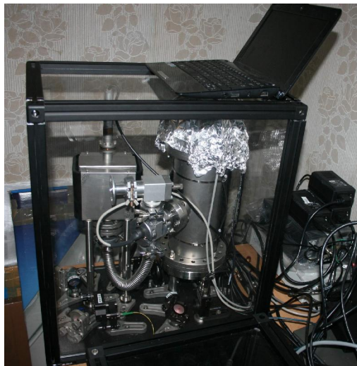
Picture 3. Temperature-stabilized Fabry-Perot resonator inside a vacuum chamber
