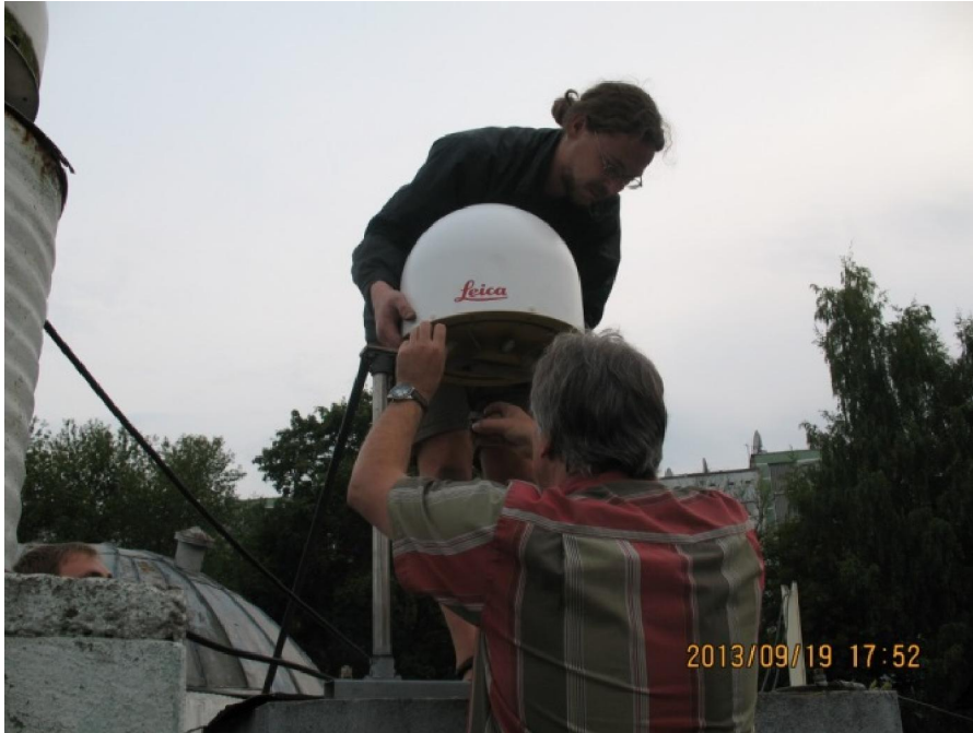
Picture 30. Installing calibrated GNSS antenna at SLR station Riga
