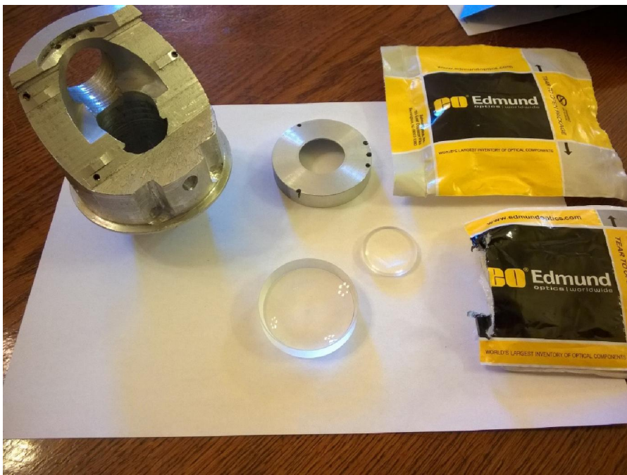
Picture 31. Optical components for the SLR system visual tracking/receiver channel unit
