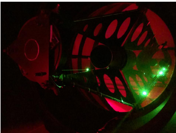
Picture 28. CPS532 laser diode during receiver channel performance evaluation
