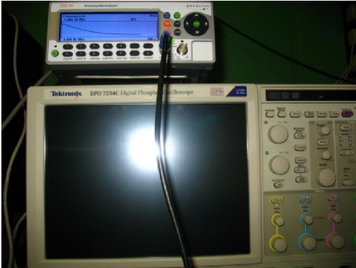
Picture 18. SLR (Satellite Laser Ranging) station test and measurement equipment: Frequency counter and analyzer Pendulum CNT-91
