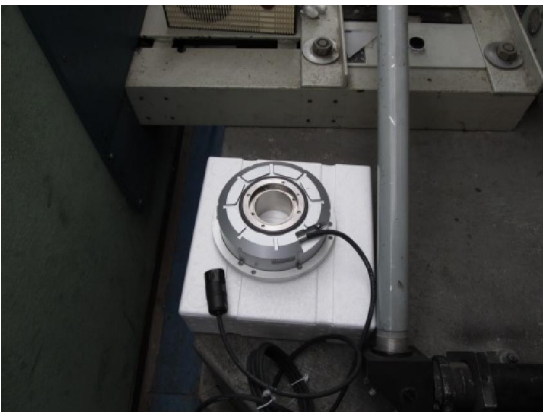
Picture 19. Heidenhain angular encoders for SLR telescope mount control
