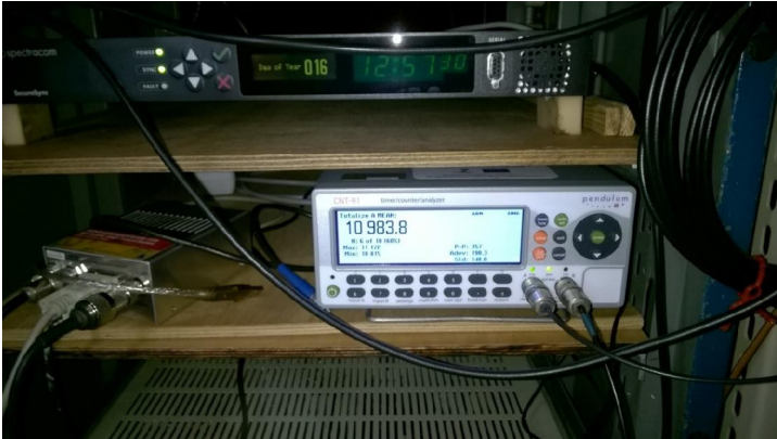
Picture 27. SecureSync auxiliary time and frequency source with OXCO together with CNT-91 counter at telescope building while testing PMT and Constant Fraction Discriminator Tennelec 456 setup
