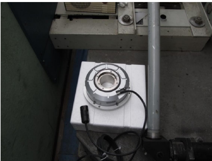
Picture 29. Encoder for telescope azimuth axis before installing within telescope
