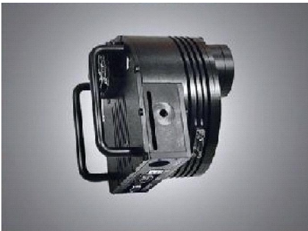
Picture 32. CCD 2184 x 1472 pixels, Size of pixel 6,7 x 6,7 \mu
