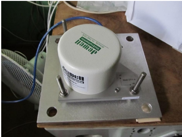
Picture 24. Jewell Instruments tiltmeter D711, measurement accuracy 1 microradian, for monitor laser ranging telescope vertical axis orientation and mount stability
