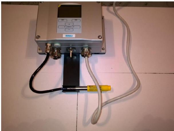
Picture 25. Vaisala PTU301 pressure, temperature and humidity sensor before installation at SLR telescope building
