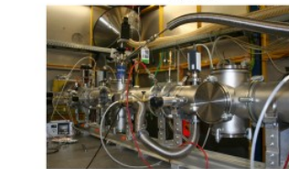
HASYLAB DESY C1 beamline XAFS experiment with He cryostat.
