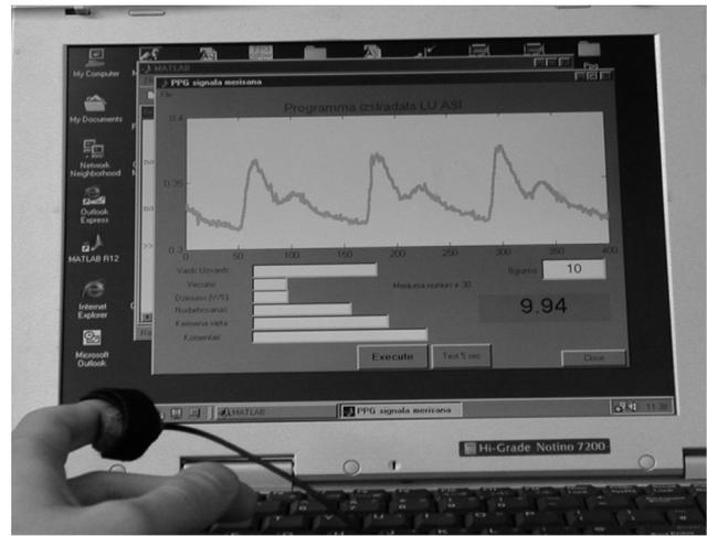
Fig. 1. Portable version of single-channel PPG sensor: application for the fingertip monitoring.
