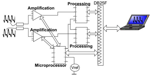
Fig. 2. Dual-channel PPG sensor device: functional scheme.
