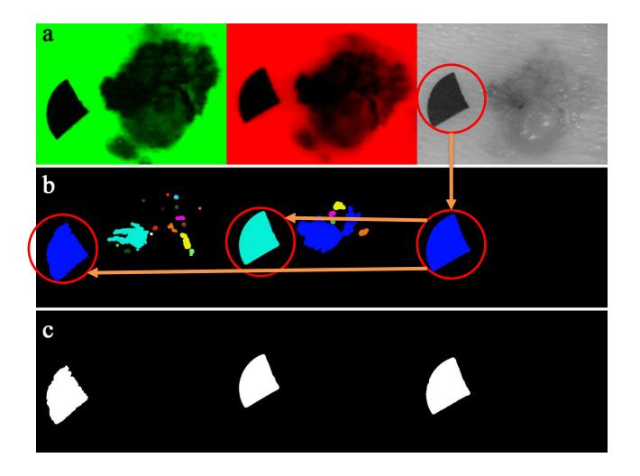
Problem: all three different multispectral images are acquired using one device, but during the process of capturing the images the device may be moved slightly, resulting in distorted positions of the three multispectral images.
