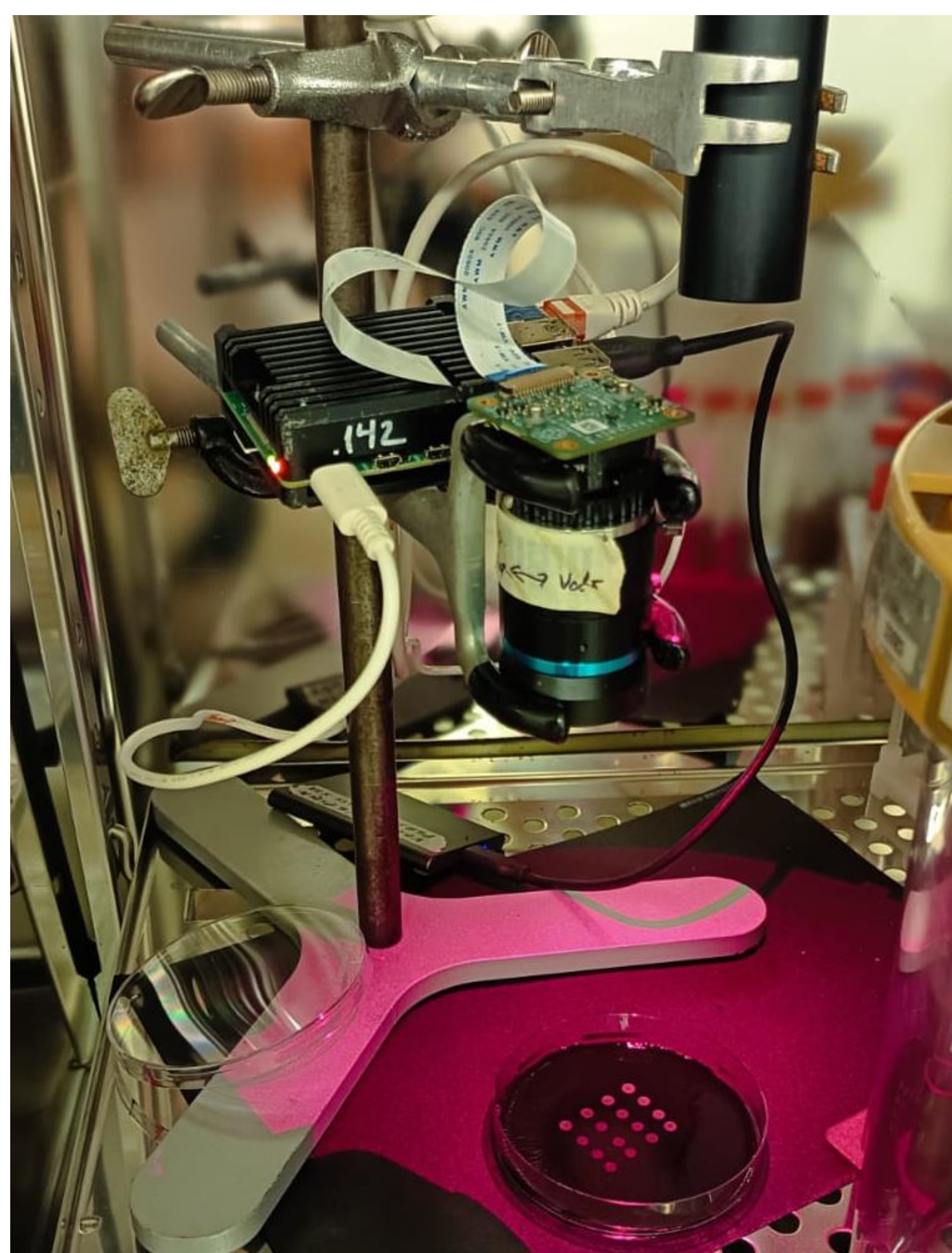
Fig. 2. Experimental setup comprising a 660 nm single-mode laser for uniform sample illumination and a 12.3 MP CMOS camera for capturing microbial growth dynamics.
