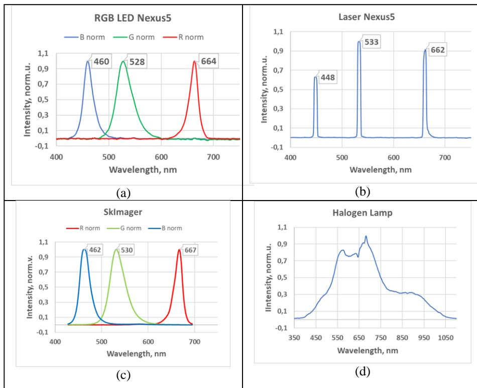
**Fig.1.** Normalized spectra of the light sources for multispectral imaging (halogen lamp - without detector sensitivity correction).
