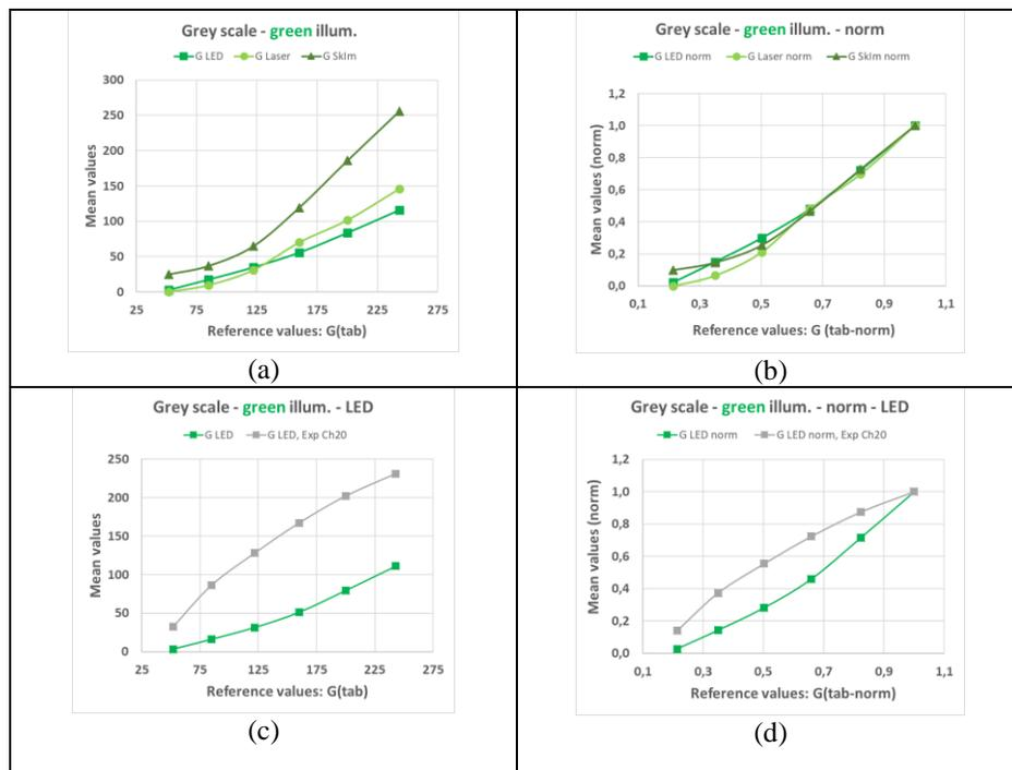
**Fig.2.** Dependences of the mean (a,c) and normalized (b,d) values on the reference values for grey scale squares of the color checker. **G** – green channel; **LED** – RGB LED illuminator; **Laser** – laser illuminator; **SKIm** – SkImager, **Exp Ch20** – exposition adjusted to the value of the square (Ch20) of the color checker, **norm** – normalized data.
