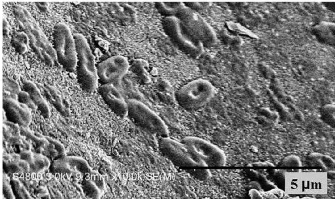
Scanning electron micrographs of the surface of ceramic beads with bacteria cells
