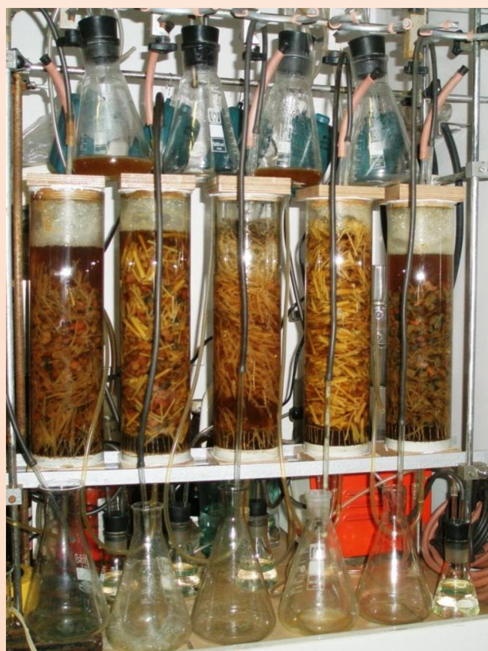
Fig.2. The five-columns biofiltration model system filled with packing material.
