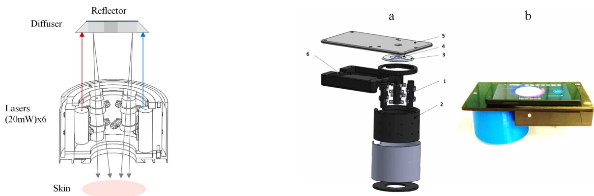
Fig. 1. Optical scheme of the 3-wavelength laser add-on illuminator (left), its design scheme (right, a) and the mobile prototype with smartphone on it (right, b): 1 – laser modules (3 pairs, 448-532-659 nm), 2 – shielding cylinder, 3 – collector of laser beams, 4 – flat ring-shaped light diffuser, 5 – sticky platform for the smartphone, 6 – electronics compartment.
