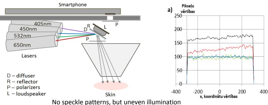
WO 2018/177565 A1, 2018. Device for speckle-free imaging under laser illumination (U.Rubins, E.Kviesis-Kipge, J.Spigulis)
