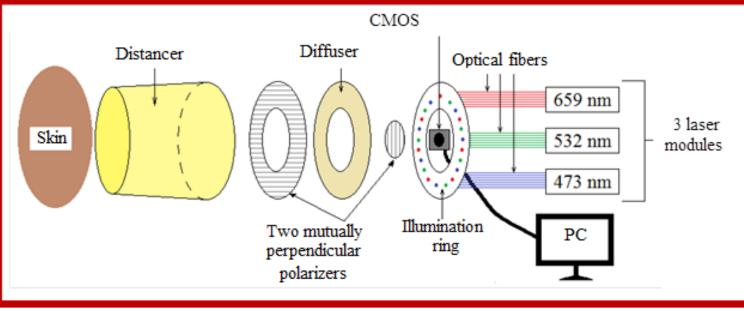
Acceptable uniformity of target illumination; drawback - too bulky, inconvenient for out-of-lab use
