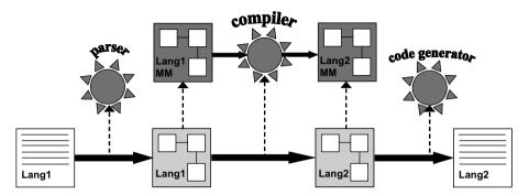
Fig. 7. Model-driven compiling – general architecture
