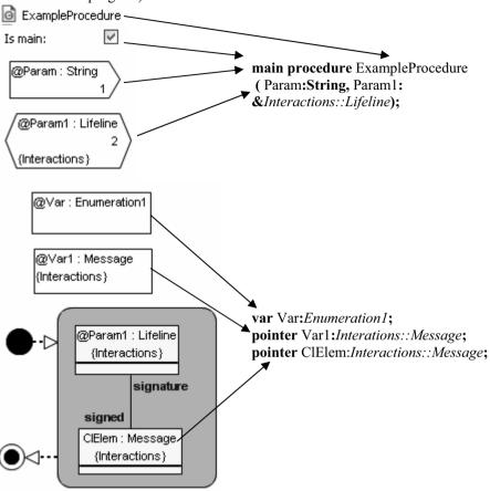
Fig. 9. Procedure header to L3
