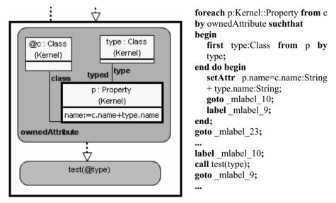
Fig. 14. The compilation of the loop
