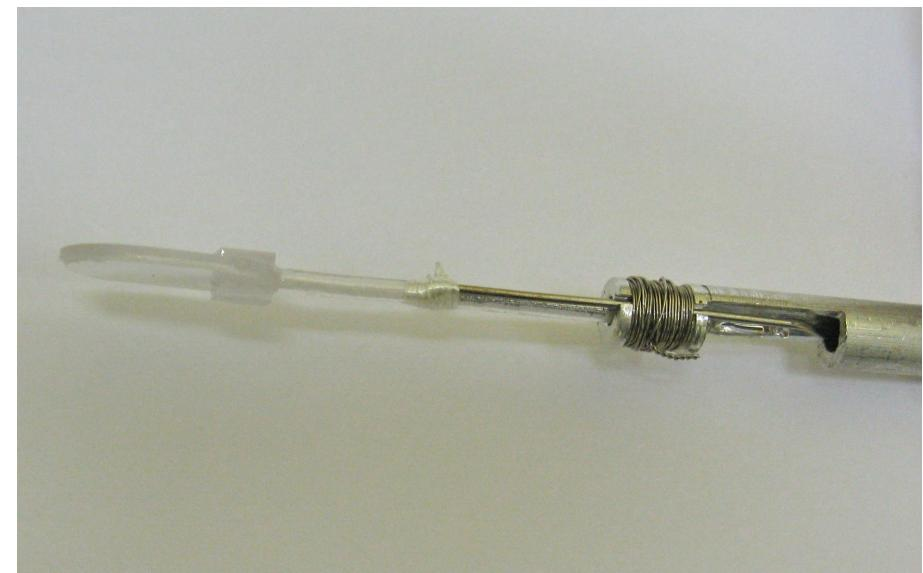
In an ETC, atoms are confined between walls separated by a distance on the order of the light wavelength, which makes possible sub-Doppler resolution. It was developed at the Institute for Physical Research in Ashtarak, Armenia.
