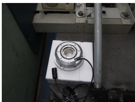
Picture 8. Heidenhain angular encoders for SLR telescope mount control
