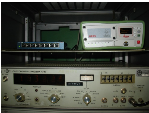
Picture 12. Geodetic GNSS receiver Leica GR25 capable of tracking all major GNSS systems: GPS, Glonass, Galileo, Beidou installed at Geodynamical station Riga
