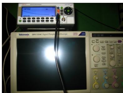
Picture 7. SLR (Satellite Laser Ranging) station test and measurement equipment: Frequency counter and analyzer Pendelum CNT-91
