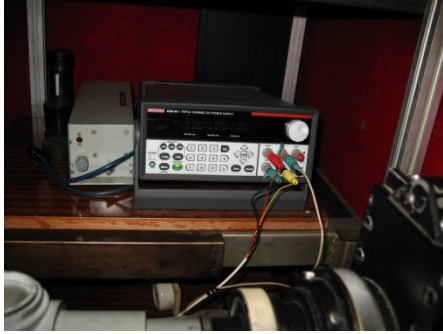
Picture 10. High stability Tektronix/Keithley DC power supply for Hammamatsu PMT photon detector installed at SLR system
