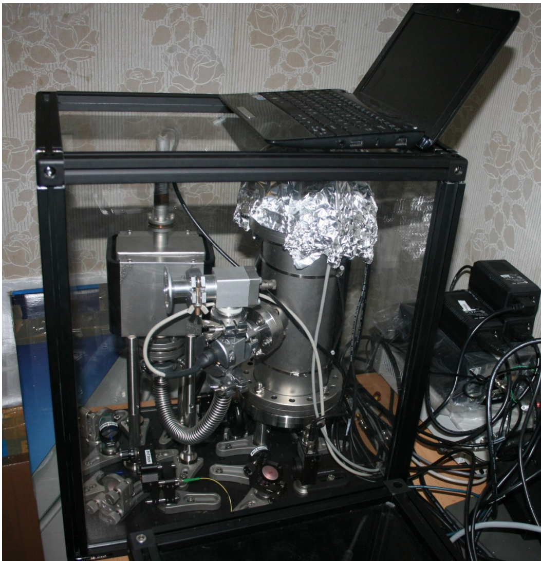
Picture 2. Temperature-stabilized Fabry-Perot resonator inside a vacuum chamber
