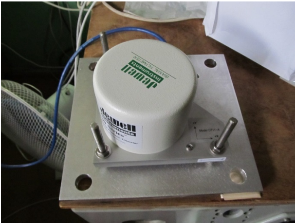
Picture 13. Jewell Instruments tiltmeter D711, measurement accuracy 1 microradian, for monitor laser ranging telescope vertical axis orientation and mount stability
