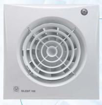
Model provided with a PIR (passive infra-red) detector. The unit starts automatically when a movement is detected within a maximum distance of 4 meters from the fan. They are also fitted with an adjustable "run on" timer, from 1 to 30 minutes, to allow the fan continues operating after the initiation of the movement detection.
