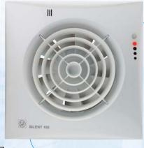
Models provided with an electronic humidistat which can be adjusted to 60, 70, 80 or 90% HR using a key situated on the front grille. Four luminous indicators show the desired level of humidity. The extractor operates automatically when the humidity level in the room is higher than the set level. The extractor will stop automatically when the humidity drops below the selected level and after the selected period set on the adjustable timer (1 and 30 minutes).
