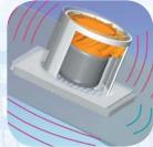
**Usual extractor** In usual extract fans the vibrations are transmitted to the surrounding areas while in SILENT extractor fans the vibrations are absorbed by
